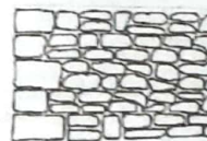
Fig. 5.15 coursed random rubble masonry
