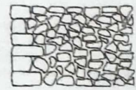
Fig. 5.16 uncoursed random rubble masonry
